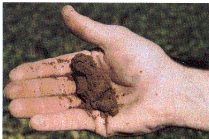
25 to 50 PERCENT AVAILABLE MOISTURE: From somewhat crumbly and non-pliable, to material which almost balls under pressure, but breaks easily, will not ribbon.
