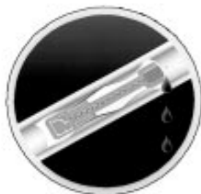
Figure 3. Cutaway example driptape emitter.
