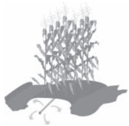
Figure 1. Dripline placement relative to corn rows in studies at the Northwest Research and Extension Center, Colby, Kansas.
