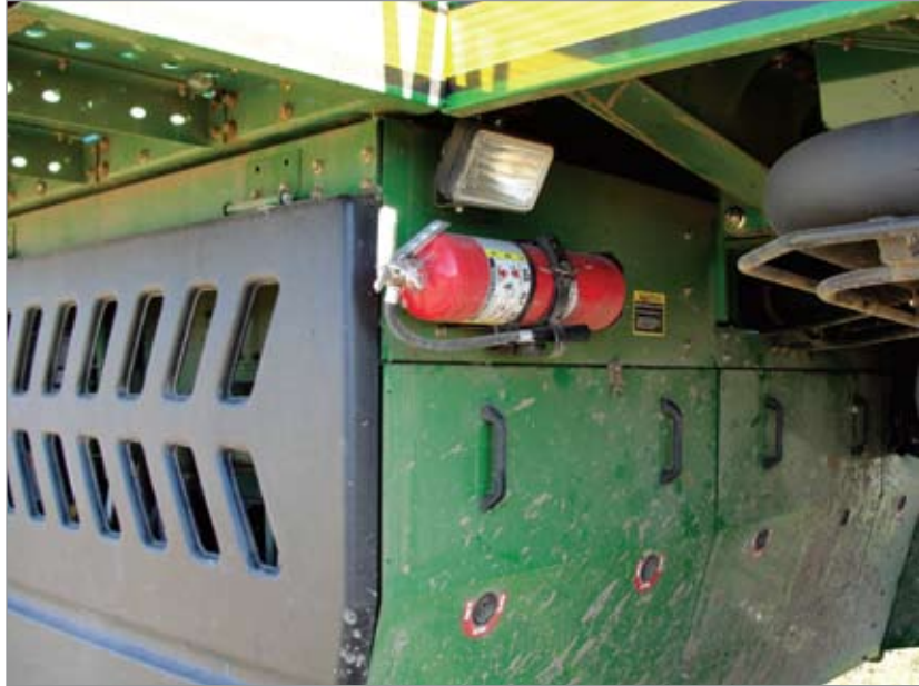
Engine compartment type ABC fire extinguisher.
