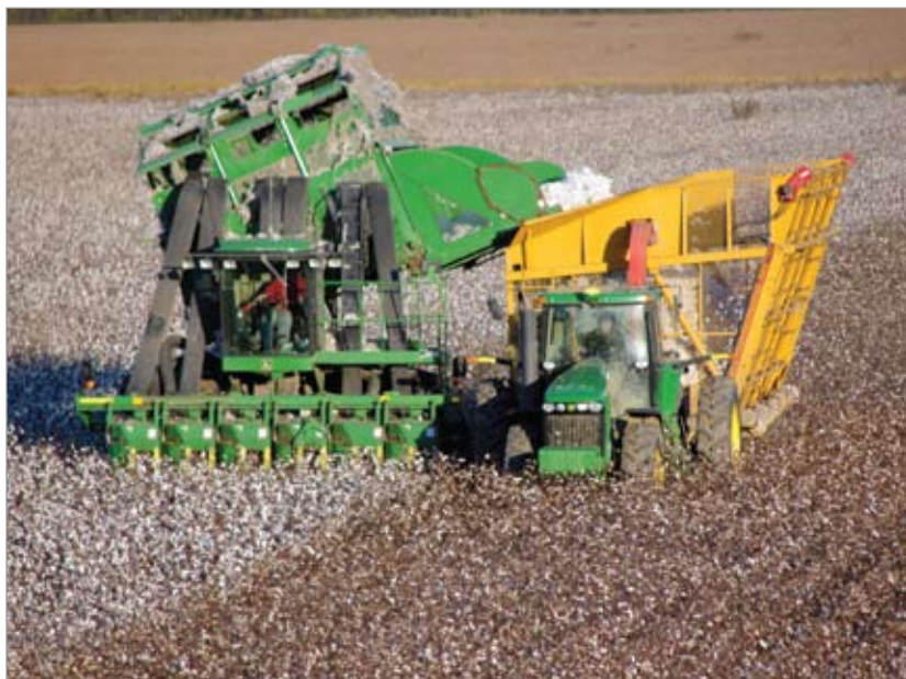
Conventional basket picker stops on the row and unloads into a boll buggy for greatest field efficiency (about 70% of time actively harvesting).
