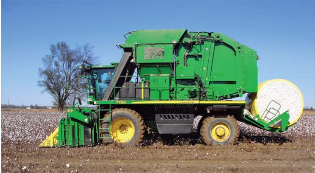
John Deere round-module-building picker carries a module before unloading while picking to the end of the row.
