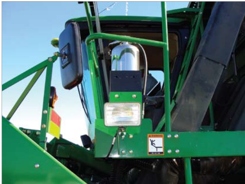
Platform water-based fire extinguisher.
