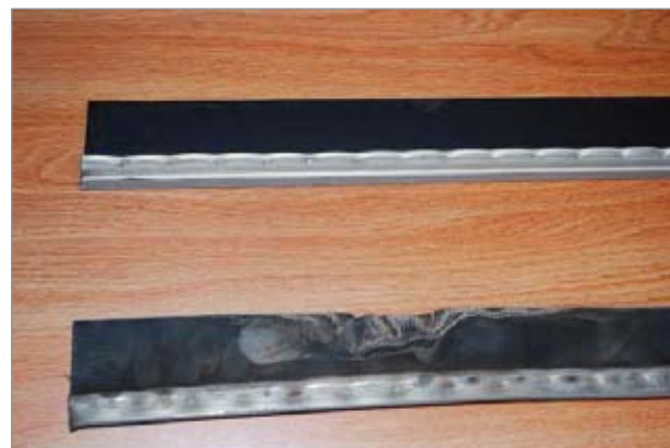
New bat (top) and worn bat (bottom).
