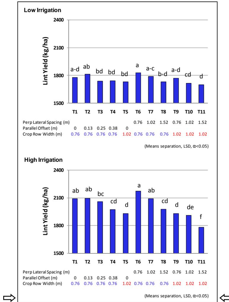
Figure 3. Average cotton lint yields from eleven crop row / drip lateral orientation treatments irrigated by SDI at low and high irrigation levels, Texas AgriLife Research, Halfway, TX, 2006-2009.
