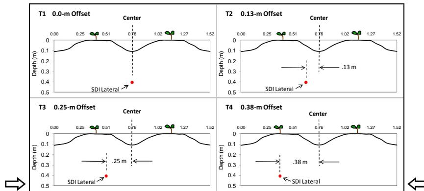
Figure 1. Illustration of treatments having row offsets from their optimum position relative to SDI laterals of 0.0, 0.13, 0.25, and 0.38 m, Texas AgriLife Research, Halfway, TX, 2006-2009.
