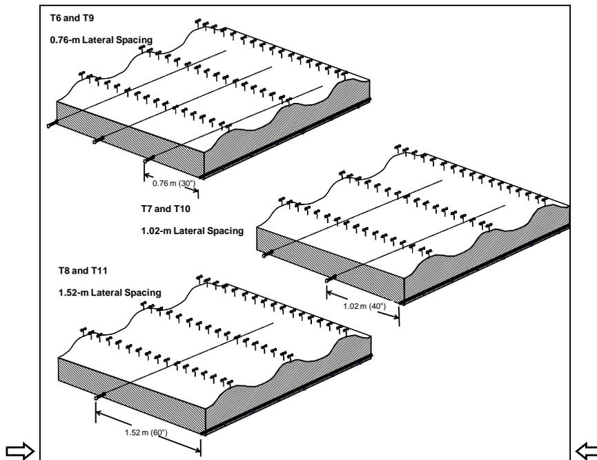
Figure 2. Illustration of three treatments with crop rows crossing SDI laterals with lateral spacings of 0.76, 1.02, and 1.52 m, Texas AgriLife Research, Halfway, TX, 2006-2009.
