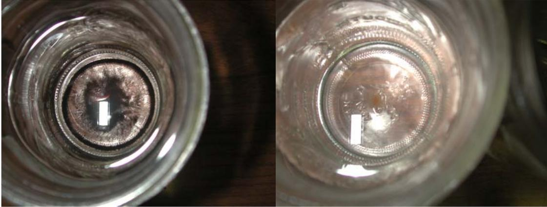
Figure 2. Two jars containing Mn at 0.04 g material/L of irrigation water, both at 0.125% H<sub>2</sub>O<sub>2</sub> concentration. The pH of the container on the left was 7.6; the pH of the container on the right was 6.5. The right jar had no visible Mn compound.
