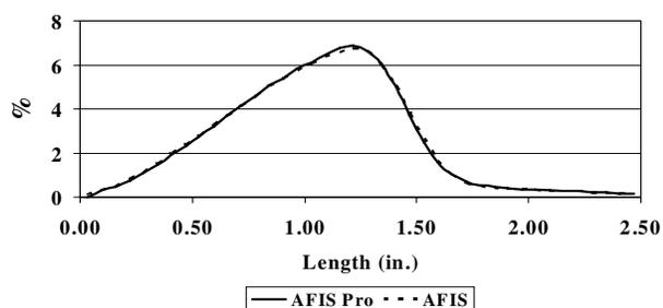
These results clearly show that fiber length distributions vary for different cottons and that the distributions are repeatable. Therefore, it is a strong hypothesis that length distributions are heritable, which would mean that varieties with superior length distributions could be developed using traditional selection techniques of plant breeders.
