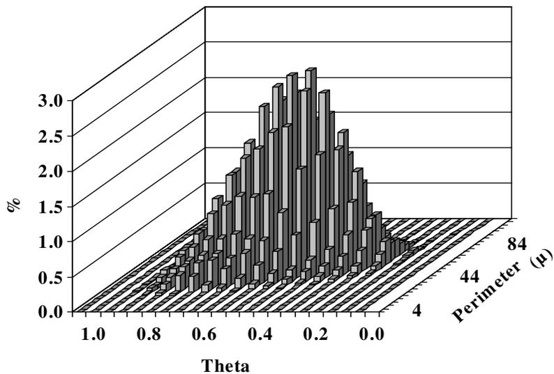
Figure 2. Bivariate Distributions of Perimeter Versus Theta, for Two Cottons with the Same Micronaire Value of 4.28
