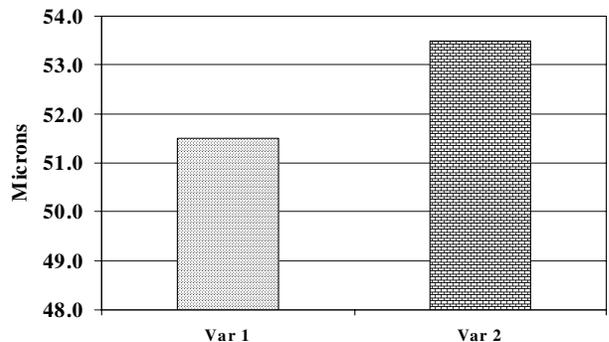
Figure 8 shows HVI upper half mean length (UHML), AFIS means length by number (ML), and AFIS short fiber content by weight (SFC(w)). Variety 1 has a significantly longer UHML; however, Variety 2 has a significantly longer ML. Furthermore, Variety 1 exhibits a much higher SFC(w). Based on measurements like these, the expectation is that Variety 2 will perform much better in ring spinning.
